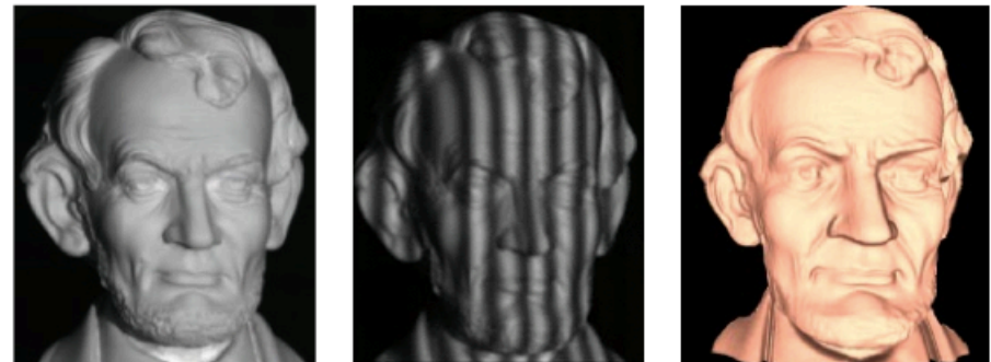
Phase-shifting [Zhang et al. 2004]
