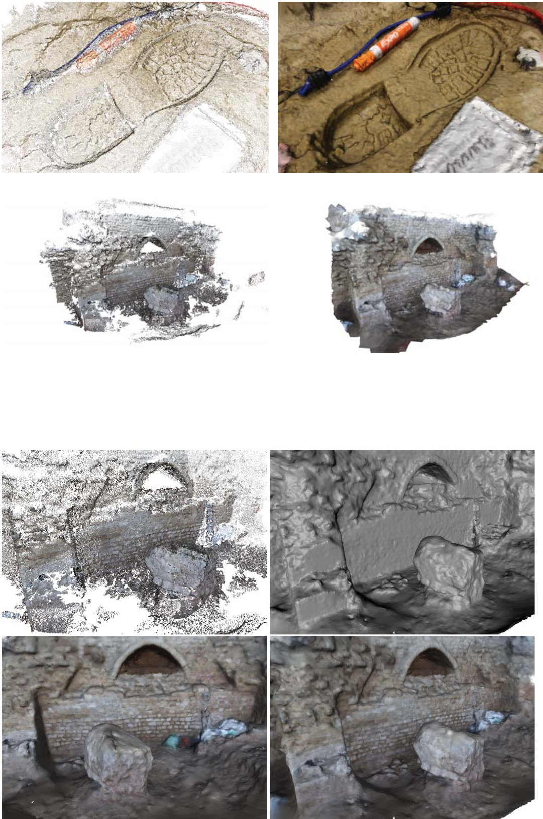
Fig. 1 Reconstruction of the side of a castle model: The input point cloud (top-left), Surface reconstructed by the proposed algorithm (top-right), Two views from the surface and color map reconstructed by the proposed algorithm (bottom).
