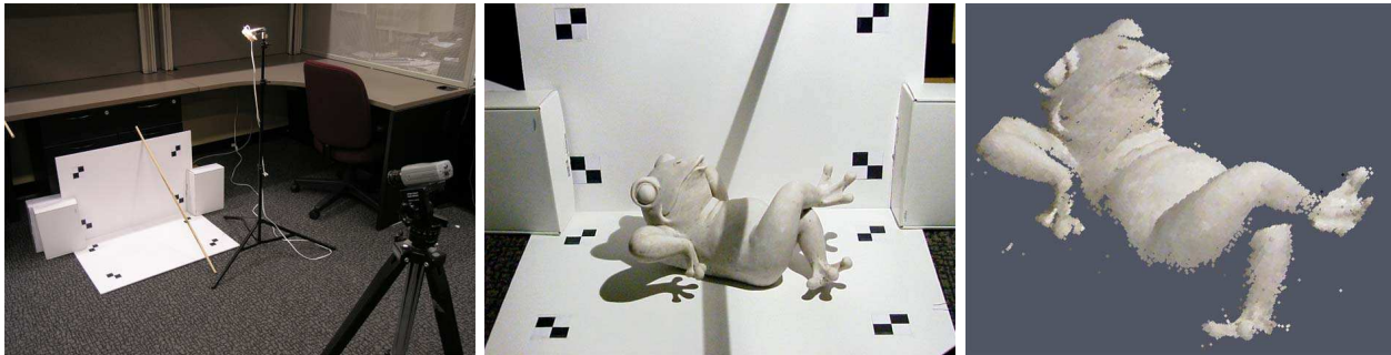
Figure 1: 3D Photography using Planar Shadows. From left to right: the capture setup, a single image from the scanning sequence, and a reconstructed object (rendered as a colored point cloud).
