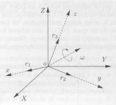
Figure 2.4. Rotation of a rigid body about a fixed point o and along the axis  $\omega$ . The coordinate frame W (solid line) is fixed, and the coordinate frame C (dashed line) is attached to the rotating rigid body.
