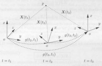
Figure 2.6. Composition of rigid-body motions.  $X(t_1)$ ,  $X(t_2)$ ,  $X(t_3)$  are the coordinates of the point p with respect to the three camera frames at time  $t = t_1, t_2, t_3$ , respectively.
