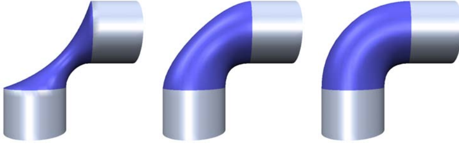
Figure 2: The order k of the energy functional defines the stiffness of the surface in the support region and the maximum smoothness C^{k-1} of the boundary conditions. From left to right: membrane surface ( k = 1 ), thin-plate surface ( k = 2 ), minimal curvature variation ( k = 3 ).
