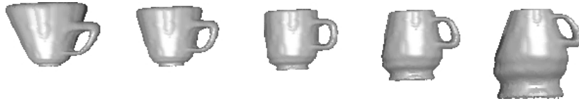
Fig. 5. Projective ambiguity: With no information about the camera or scene, there is a 1D projective ambiguity in the z direction. Five models of the cup with different choices for \mathbf{h}_3 .
