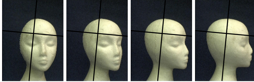
Fig. 4. Fixed image lines. The fixed image lines are shown overlaid on images from the head sequence. The almost vertical line is l_s , the horizontal line is l_h (see also figure 3a). The eyebrow of the mannequin, which is approximately coplanar with \pi_h , remains tangent to l_h as the object rotates. These fixed lines are automatically computed from the images using the algorithm of §3.
