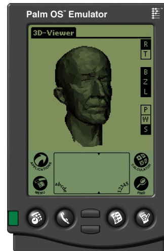
Figure 31: Low-polygon approximation (2k triangles) of the Max Planck bust (~400k triangles, see Figure 9) on the PalmPilot PDA
