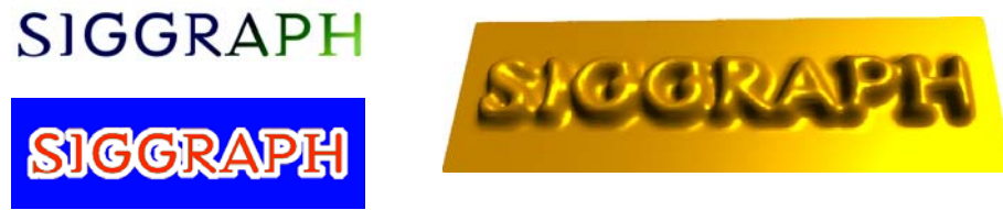
Figure 6.13 Embossing effect. The Siggraph label on the top left has been converted to a selection stencil using simple image processing tools. This stencil can then be mapped to a surface, where blue color corresponds to the zero-region and red to the one-region. Subsequent deformation yields an embossing effect as shown on the right.
