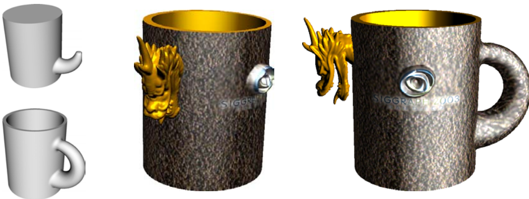
Figure 8.6 Creating a coffee mug using boolean operations, deformation, collision detection and particle-based blending. [see Color plate 8 on page 131]
