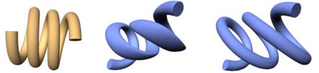
Figure 3: A SPRING is deformed using a spatial deformation technique (center) and our method (right). In the spatial case, points in close proximity (Euclidean metric) move together even when their geodesic distance is much larger. In contrast, our mesh-based approach contains this geodesic information implicitly.
