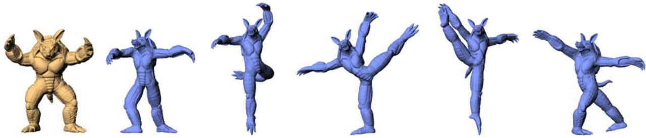
Figure 7: This figure shows the initial ARMADILLO mesh followed by a few frames from the ballet sequence. The entire volume graph has 525K free vertices and the running time is 2.88 seconds/frame. Combining the 20 rotation constraints at each vertex requires a non-negligible portion of the per frame time. These results were generated by our solver at an accuracy of < 1e-3 relative residual.
