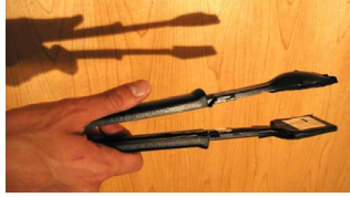
These three-dimensional digital tongs contain a 6-DOF sensor in their base. A contact switch detects when they are closed. These tongs are used to move and stretch shapes in the surface drawing system.
