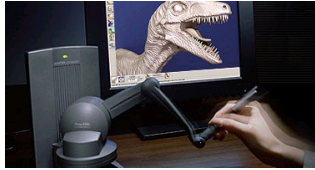
The phantom input device controls the deformation of the onscreen model. Through haptic feedback, the user can feel the surface as it is deformed.
