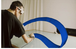
The path of the hand in space is rendered as a geometric object. The curvature of the hand defines the curvature of the stroke: a large amount of data is specified in each sweep of the hand.
