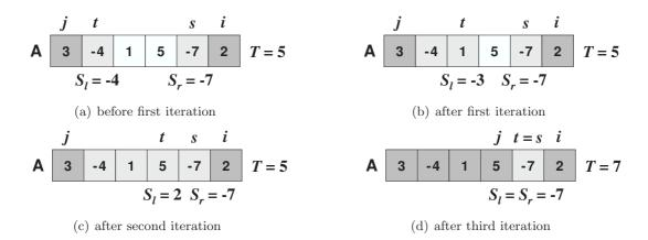
Figure 2: Operation of MAX-CYCLIC-SUBARRAY. The state of the maximum cyclic subarray estimate is shown in (a) through (d), where the shading corresponds to the the state of the array element. White indicates that the element has not yet been considered. Light gray indicates that the element has been added to either the  $S_l$  or  $S_r$  accumulators. Dark gray indicates elements that are part of the current MSS estimate. Note that the final output is found after three iterations.
