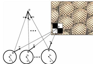
Illustration of bundle adjustment using a planar calibration target. (Features are manually selected.)
