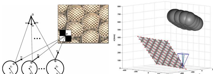
Illustration of bundle adjustment using a planar calibration target.
