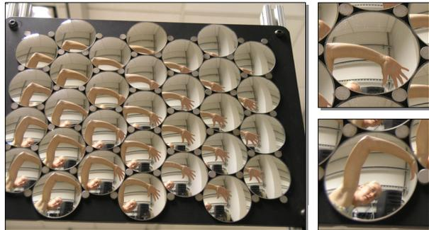
Typical image captured by the Olympus 8 megapixel digital camera. Images from individual mirrors demonstrate the wide field of view.
