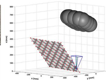
Calibration results using a checkerboard. Red circles represent the reconstructed positions of the checkerboard corners.
