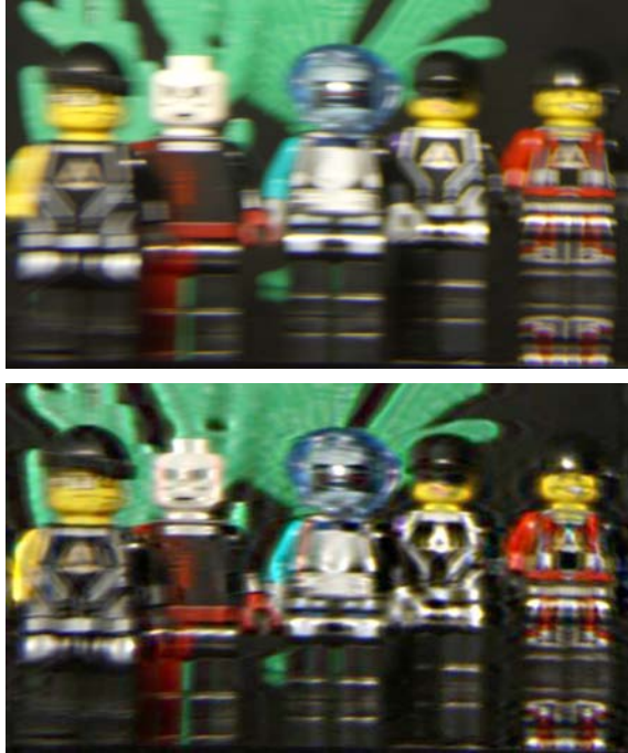
Figure 9. Depth-invariant blur size. (Top) We create a depth invariant blur size by focusing a lens with a horizontal slit aperture close to the camera, and create a virtual focal plane farther in the scene using image destabilization. The PSF produced by both forms of defocus is very similar and the overall result is an approximately depth invariant defocus kernel. (Bottom) Although the overall PSF is not strictly invertible, Richardson-Lucy deconvolution provides reasonable results for an approximate all-in-focus image.
