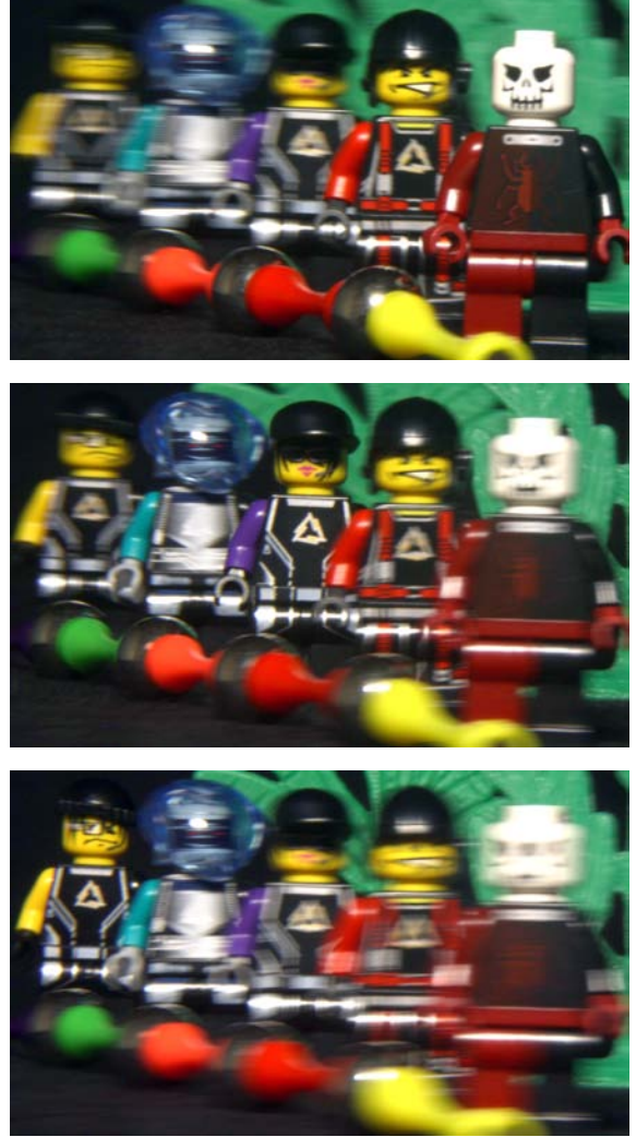
Figure 6. Reduced depth of field using image destabilization and a physical aperture of f/22 . (Top) Focused on the front figure with t_p = 10mm , (Middle) focused in the middle with t_p = 5mm , and (Bottom) focused in the back with t_p = 10mm . The relative translation velocities are adjusted according to Equation 1 to focus at various planes in the scene. The f-number reduces with increasing lens translation range, t_p .
