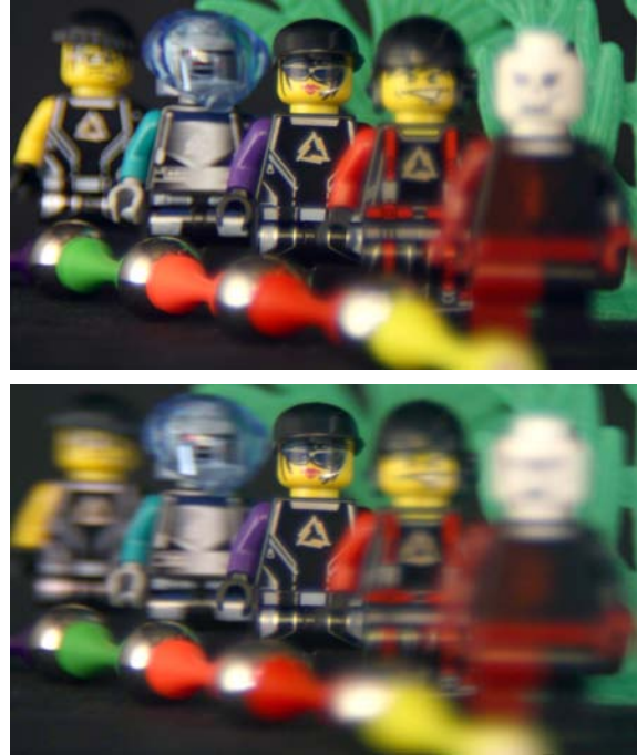
Figure 8. Reducing the depth of field using image destabilization. (Top) A photograph taken with a static lens with an f/2.8 aperture (Bottom) Synchronized translation of the lens and sensor simulates the effect of a larger virtual aperture. The depth of field is shallower, and the bokeh is visually more pleasing both in front of and behind the plane of focus.
