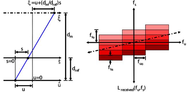
**Figure A.2:** Geometric derivation of tiled-broadband mask separation. (Left) The two-plane parameterization  $(u, s)$  of the optical ray shown in blue. The ray intersects the mask at  $\xi = u + (d_m/d_{ref})s$ . (Right) The received light field spectrum contains multiple spectral replicas shown in shades of red. The shield field spectrum must lie along the dashed line (i.e.,  $f_s/f_u = (d_m/d_{ref}) = f_{sR}/(2f_{u0})$ ).
