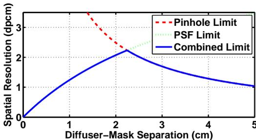
**Figure A.1:** Effective spatial resolution as a function of diffuser-mask separation  $d_i$  for a pinhole array, as given by Equation 4. System parameters correspond with the prototype in Section 6.1.
