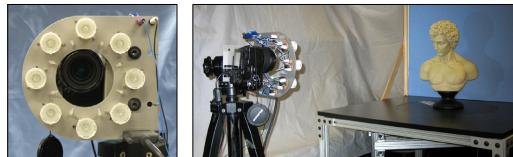
*Acquisition hardware: An Olympus C-8080 8 megapixel digital camera with 8 LED flashes and a computer-controlled turntable.*
