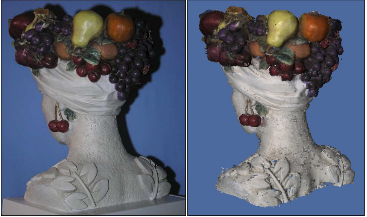
Figure 2: Reconstruction results for the woman with fruit basket model. On the left, an image acquired with the flash located to the left of the camera. On the right, the point-based reconstruction using 67 images to estimate the Phong reflectance model.
