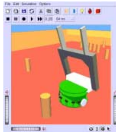
Fig.1a: Close up of a simulated robot (5.5 cm in diameter) in Webots equipped with a gripper turret in front of a seed.
