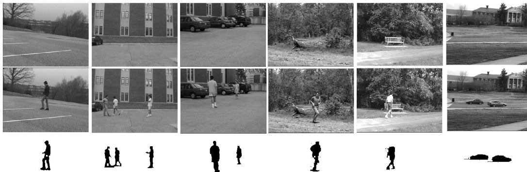
Fig. 6. An example of foreground region detection while background has different intensity variation.
