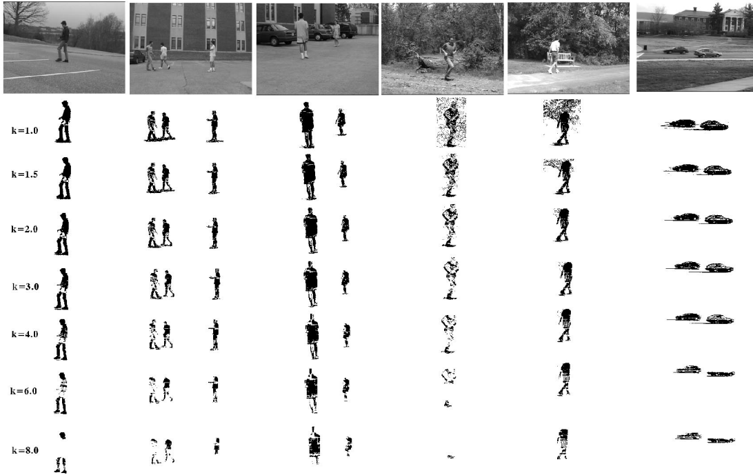
Fig. 5. An example of foreground region detection for different threshold values.
