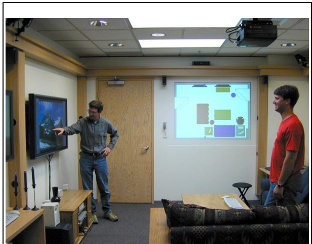
Figure 1: We track multiple people using stereo cameras in the EasyLiving lab, which is an intelligent environment set up to look like a living room.
