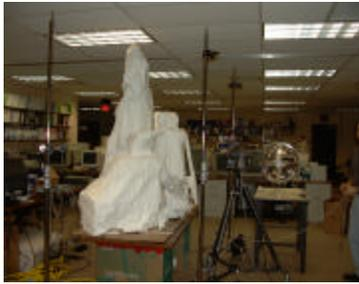
To get a basic idea of where each mesh would go, we planned to use a tracker on the camera. We knew that this alone would not be enough, because small errors in camera location and orientation would result in large error in mesh location for a camera that is about 0.75 m from the statue. To get finer alignment, we used lasers to project spots on the statue as landmarks that could be used to align the meshes.
