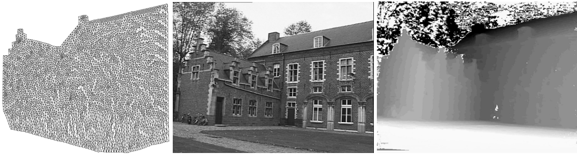
Figure 8.1: Surface reconstruction approach: A triangular mesh (left) is overlaid on top of the image (middle). The vertices are back-projected in space according to the value found in the depth map (right).
