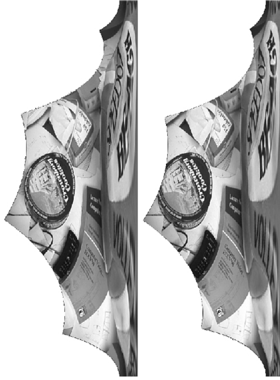
Figure 7.14: Rectified pair of images of the desk. It can be verified visually that corresponding points are located on corresponding image rows. The right side of the images corresponds to the epipole.
