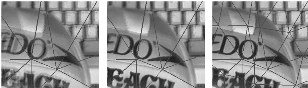
Figure 8.14: Details of rendered images showing the differences between the approaches: one global plane of geometry (left), one local plane for each image triple (middle) and refinement of local planes (right).
