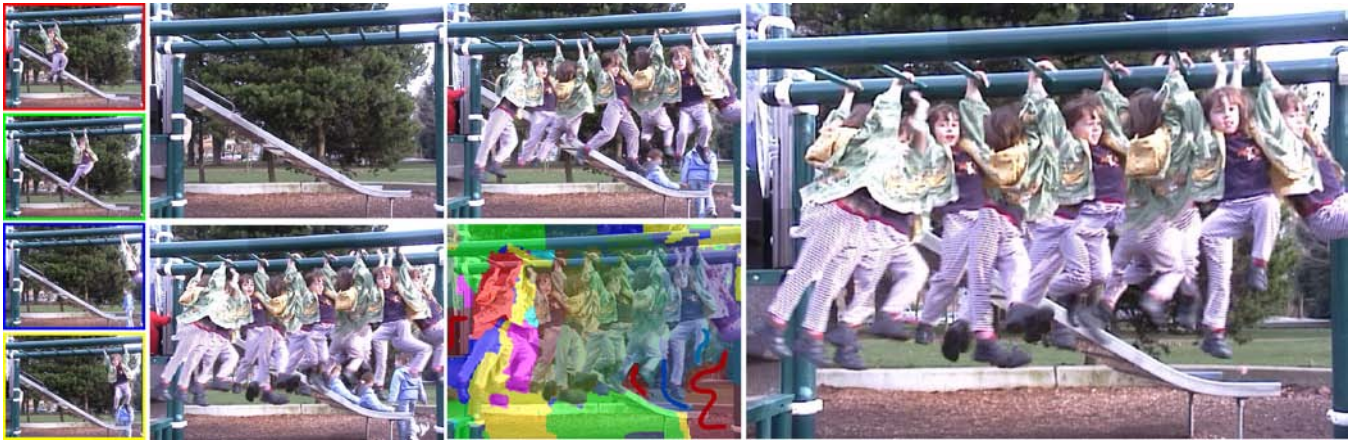
Figure 5 To capture the progression of time in a single image we generate this stroboscopic image from a video sequence. Several video frames are shown in the first column. We first create a background image using the maximum likelihood objective (second column, top) and then add it to the stack. Then, we use the maximum difference objective to compute a composite that is maximally different from the background (second column, bottom). A lower weight for the image objective results in fewer visible seams but also fewer instances of the girl (third column, top). Beginning with the first result, the user removes the other girls by brushing in parts of the background and one of the sources using the designated source objective (third column, bottom) to create a final result (right).
