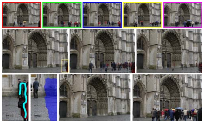
Figure 12 From a set of five images (top row) we create a relatively clean background plate using the maximum likelihood objective (middle row, left). The next two images to the right show that our result compares favorably to a per-pixel median filter, and a per-pixel maximum likelihood objective, respectively. An inset of our result (bottom row, left) shows several remaining people. The user paints over them with the eraser objective, and the system offers to replace them with a region, highlighted in blue, of the fourth input image. The user accepts this edit, and then applies gradient-domain fusion to create a final result (bottom row, middle). Finally, using a minimum likelihood image objective allows us to quickly create a large crowd (bottom right).
