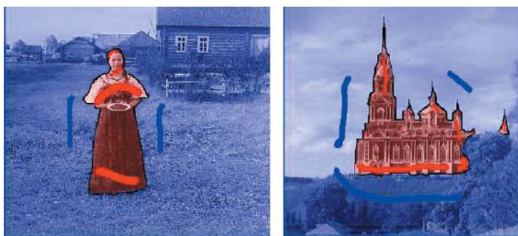
Figure 3.66: Image segmentation example (Boykov and Funka-Lea 2006). The user draws a few red strokes in the foreground object and a few blue ones in the background. The system computes color distributions for the foreground and background and solves a binary MRF. The smoothness weights are modulated by the intensity gradients (edges), which makes this a conditional random field (CRF).
