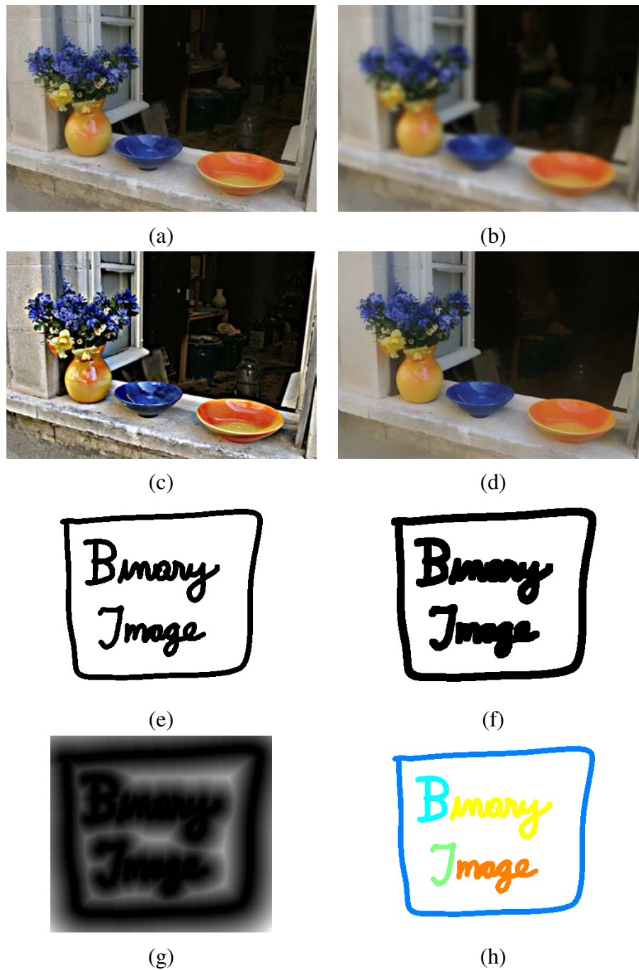
Figure 3.9: Some neighborhood operations: (a) original image; (b) blurred; (c) sharpened; (d) smoothed with edge preserving filter; (e) binary image; (f) dilated; (g) distance transform; (h) connected components. For the dilation and connected components, black (ink) pixels are assumed to be active (1).
