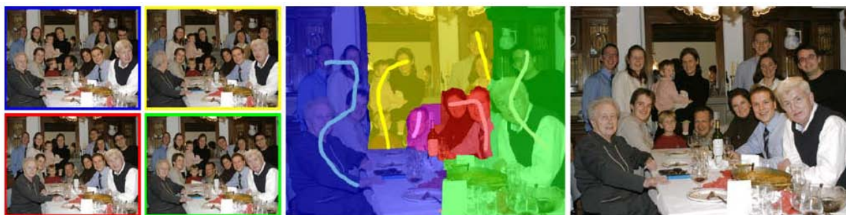
Figure 3.65: An example of an unordered label MRF (Agarwala et al. 2004). Strokes in each of the source images on the left are used as constraints on an MRF optimization, which is solved using graph cuts. The resulting multi-valued label field is shown as a color overlay in the middle image, and the final composite is shown on the right.
