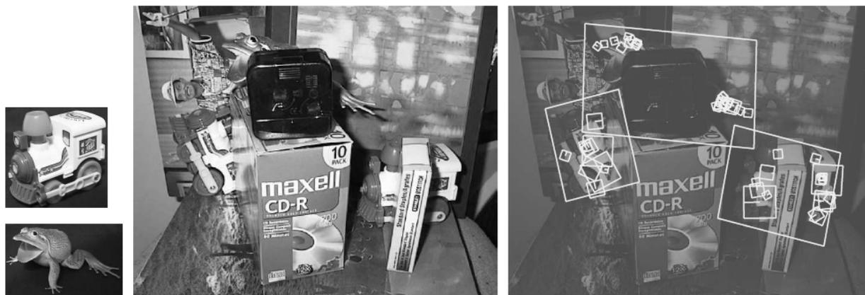
Figure 4.21: *Recognizing objects in a cluttered scene (Lowe 2004).* Two of the training images in the database are shown on the left. These are matched to the cluttered scene in the middle using SIFT features, shown as small squares in the right image. The affine warp of each recognized database image onto the scene is shown as a larger parallelogram in the right image.
