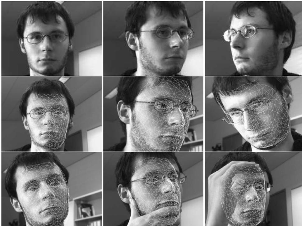
Figure 4.29: *Real-time head tracking using the fast trained classifiers of Lepetit et al. (2004).*
