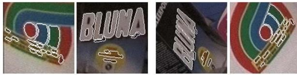
Figure 4.15: *Maximally Stable Extremal Regions (MSERs) extracted and matched from a number of images (Matas et al. 2004).*
