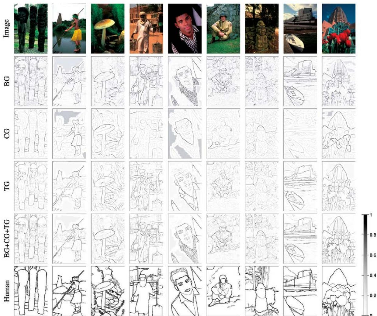
Figure 4.36: Combined brightness/color/texture boundary detector (Martin et al. 2004). Successive rows show the outputs of the brightness gradient (BG), color gradient (CG), texture gradient (TG), and combined (BG+CG+TG) detectors. The final row shows human-labeled boundaries derived from a database of hand-segmented images (Martin et al. 2001).
