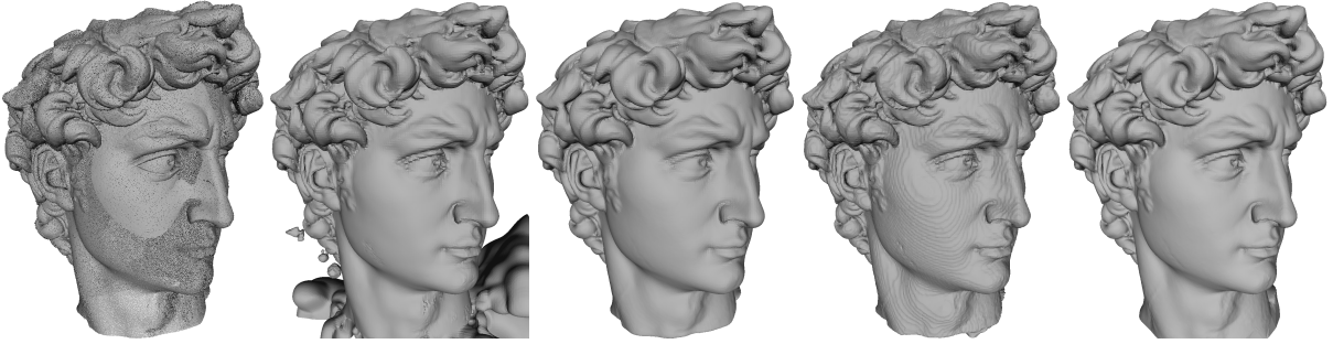
Figure 5: Input point cloud (leftmost) of David's head, and reconstructions using (from second-left to right) MPU, Poisson, D4 Wavelets, and our SSD reconstruction.
