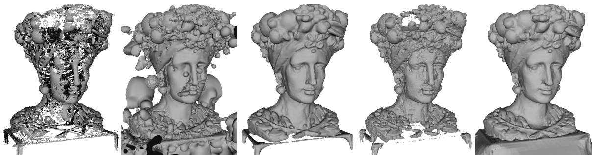
Figure 8: Input point cloud (leftmost) of the Chiquita model, and reconstructions using (from second-left to right) MPU, Poisson, D4 Wavelets, and our SSD reconstruction.
