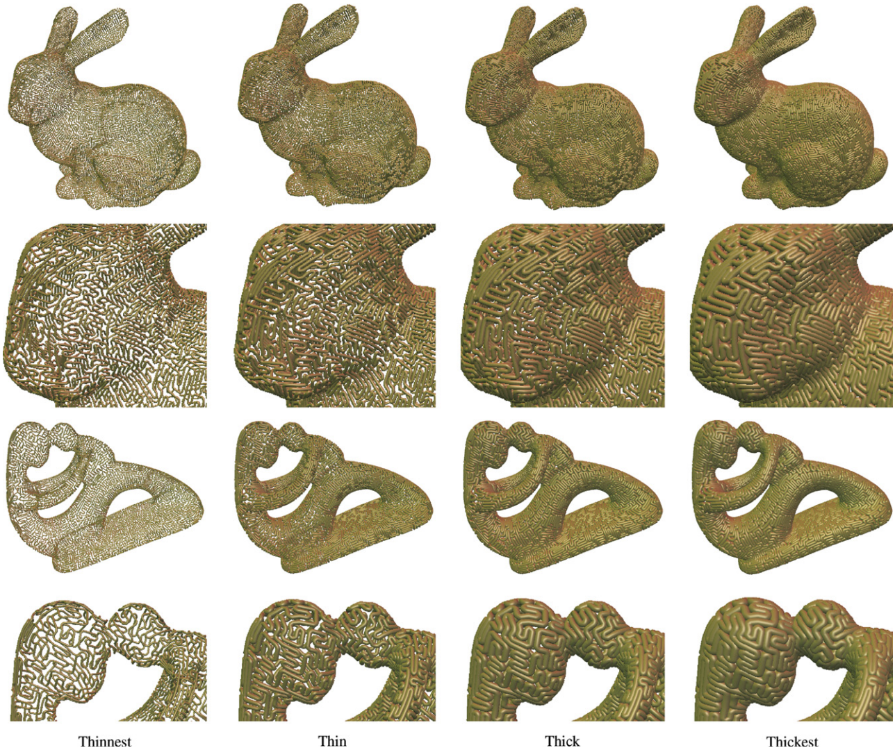
Fig. 14. Examples of quadrilateral meshes covered with constant diameter wires. Note that if all faces of the original mesh are approximately same size as in this example constant diameter method can densely cover the surface without significant self intersection. Back-face parts of the wires are shown. The original quadrilateral mesh of bunny is obtained by Quadcover method. The original quadrilateral mesh of fertility is obtained by mixed-integer quadrangulation.
