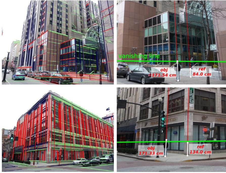
Fig. 11. Measuring the height of a person. The first column contains the input image with the segment clustering result. The second column presents a crop with the computed height.
