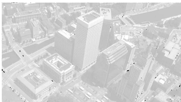
Fig. 7. Changes detected by the proposed algorithm are marked in black. Note that the moving vehicles have low probability, as well as some false detects around building edges, presumably due to small errors in the camera model. Original image courtesy of Brown University.
