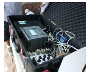
Figure 6: Permanently mounting the computers in a case simplified setup and made the connections more reliable
