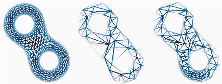
15 An example of selective refinement (the original mesh is shown on the left). The partial ordering of edge collapses and vertex splits enables a consistent subset of vertex splits (right) starting from a simplified mesh (middle).
