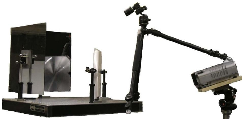
**Fig. 4.** Surround structured lighting prototype viewed from the side. Note the key components, from left to right: the first-surface planar mirrors mounted on fine-tuning gimbals, the Fresnel lens, a high-resolution digital camera, and a DLP projector mounted on a geared tripod head.
