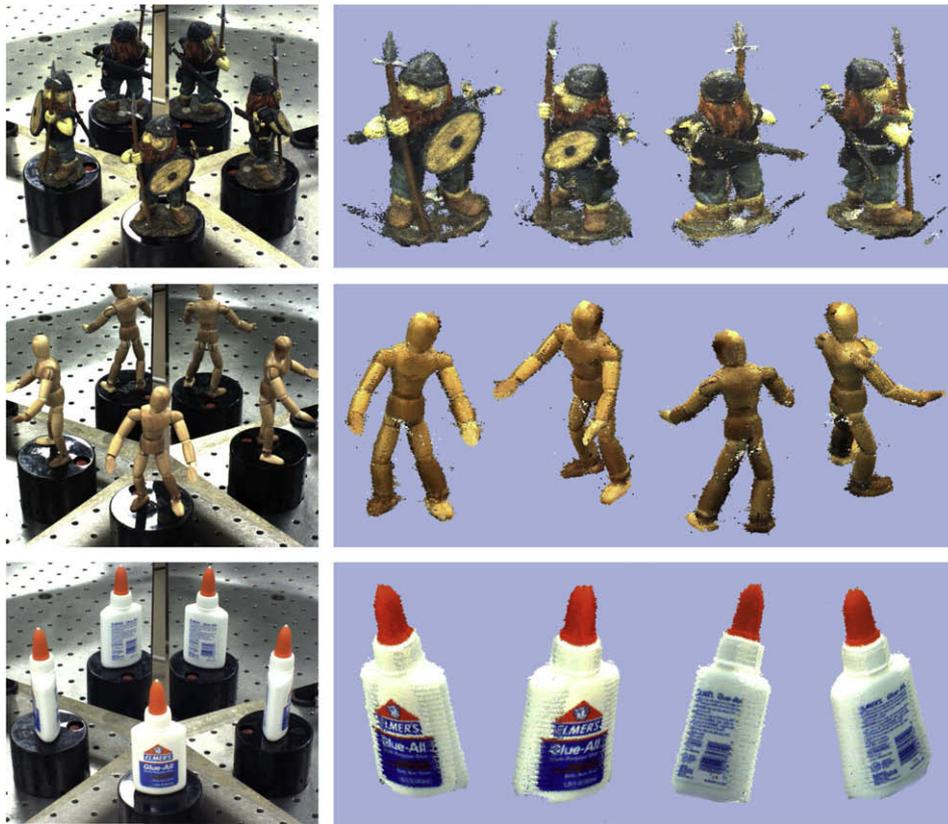
Fig. 13. Summary of reconstruction results. From left to right: the input images used for texture mapping and four views of the 3-D point cloud recovered using the proposed method with a single camera and orthographic projector.
