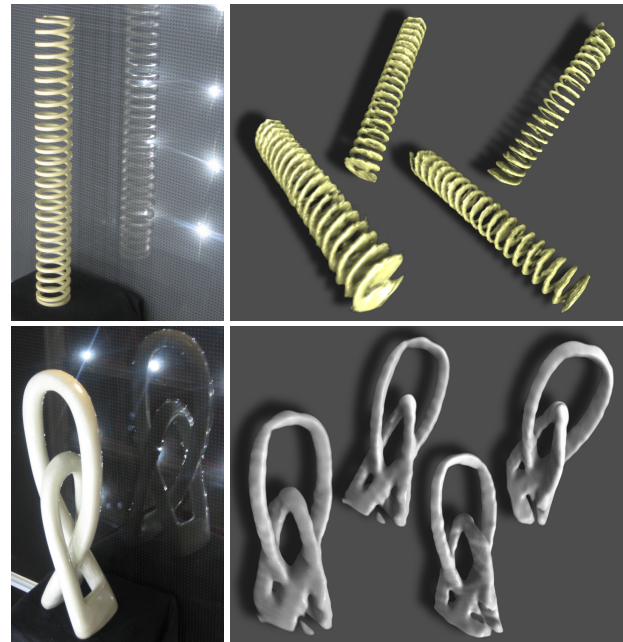
Figure 10: Visual hulls from shield fields. (Top row) A 5mm thick spring (shown with a tiled-MURA pattern) and its visual hull reconstruction. (Bottom row) A 2cm thick sculpture (shown with a tiled-pinhole pattern) and its reconstruction. The right column shows four views of visual hull (i.e., the 50%-confidence isosurface).
