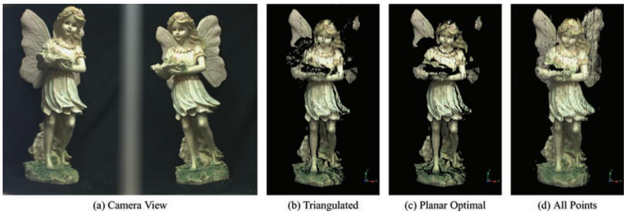
**Figure 12:** Catadioptric camera view and reconstruction results using triangulation and optimal planar projection. Points in (c) are reconstructed from both views and (d) shows the addition of points seen only from one view.
