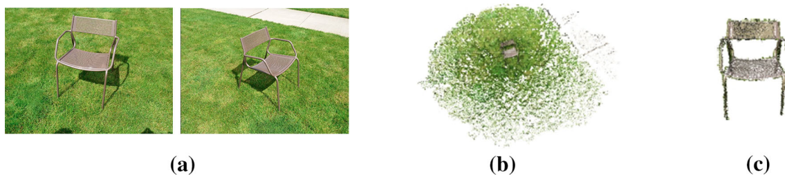
Fig. 11 Two of 41 images used in the reconstruction of a chair (a), the generated 3D point clouds (b) and segmentation result (c)
