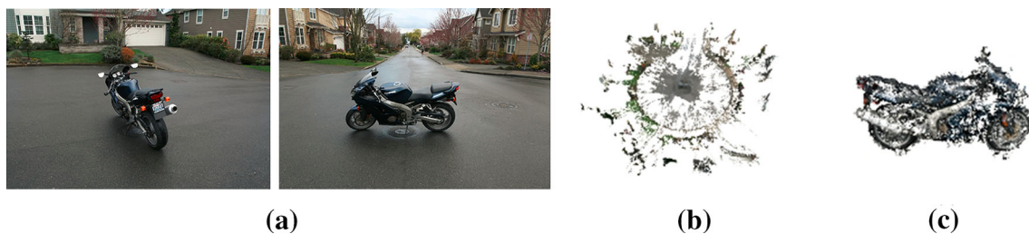
Fig. 10 Two of 35 images used in the reconstruction of a motorbike (a), the generated 3D point clouds (b) and segmentation result (c)
