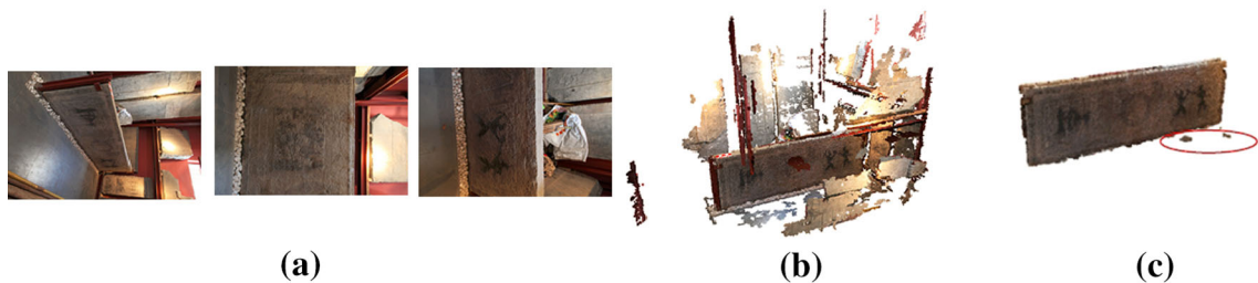
Fig. 8 Three of 79 images used in the reconstruction of a stone relief (a), the generated 3D point clouds (b) and segmentation result (c)
